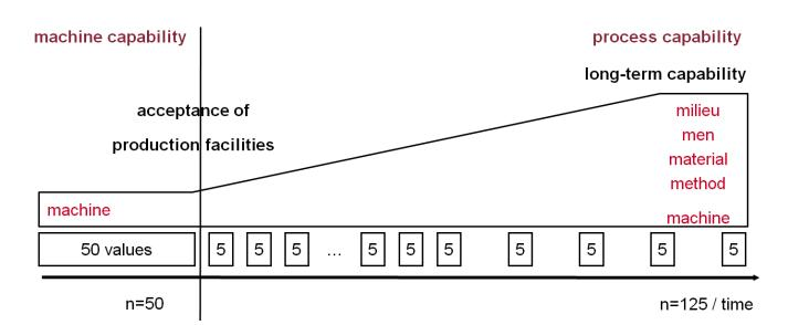
The graphic displayed above illustrates the relationship between machine and process capability. Detailed information about machine and process capability is provided in the article "Process Capability – a Simple Illustration".
