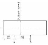
The size is a two-point size and must not exceed the tolerance interval of  $25 \pm 0.1$  in the interval from A to B where A = 20 mm.
