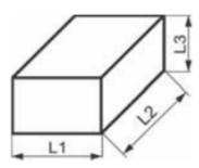
Three linear sizes (distance between two opposite planes) L1, L2 and L3 The cuboid becomes a cube when all six faces are square. In this special case, the features of size are two pairs of parallel lines, e.g. L1 and L3.
